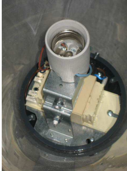
Photograph No. 5 Luminaire after IP6X (Pass no dust into luminaire )
