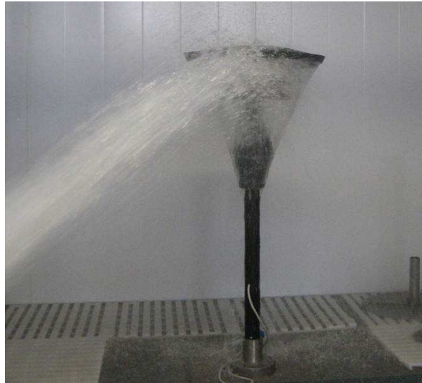
Photograph No. 7 Luminaire during IPX6 Test.
