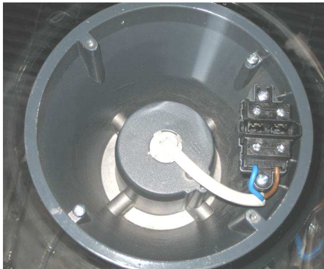
Photograph No. 14 Luminaire after IPX6 (Pass no water inside luminaire)
