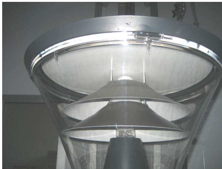
Photograph No. 10 Luminaire after IPX6 (Pass no water inside luminaire)
