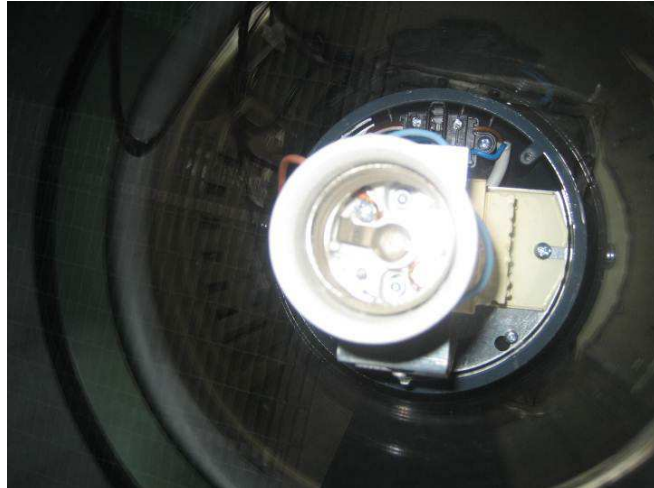
Photograph No. 13 Luminaire after IPX6 (Pass no water inside luminaire)
