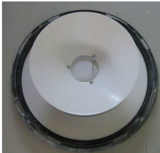
Photograph No. 6 Luminaire after IP6X (Pass no dust into luminaire )
