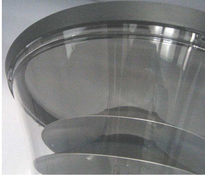
Photograph No. 9 Luminaire after IPX6 (Pass no water inside luminaire)
